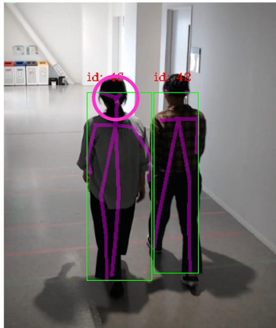
図 28 Lightweight OpenPose の認識失敗例 (0.2m)
