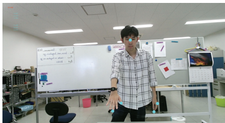
Fig. 1 Joints of a worker detected by Kinectv2.
